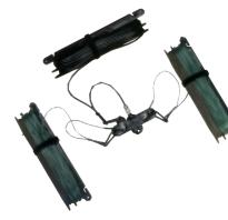
The RF-1941/RF-1940 Series are lightweight, portable dipole antennas designed for use in the 2 to 30 MHz range with a maximum power of 500 Watts. The antenna is stored on selfcontained flat spools, which form an integral part of the antenna. During operation, unwind to frequency marker and deploy; the unused portion remains on the storage spool. Each spool also contains throwing line that can be connected to masts, trees, buildings, poles, etc.
